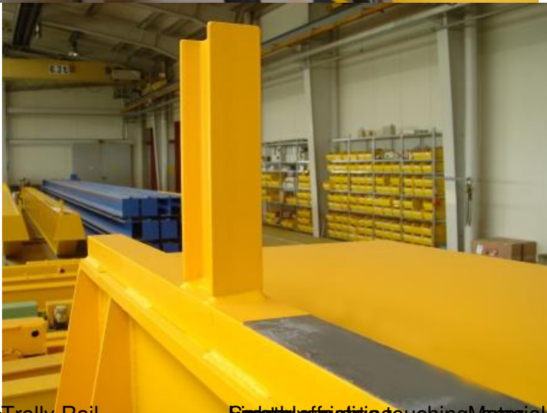
• Trolley Rail • Single high-tensile touching material: ST52 Hot rolled steel bar
