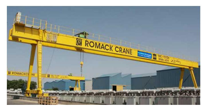
**ROMACKcrane** Gantry Cranes can be constructed with a cantilever to allow handling outside the rail centres. Typical applications for this type of crane include steel stock yards, loading areas, the concrete industry and ship building.
